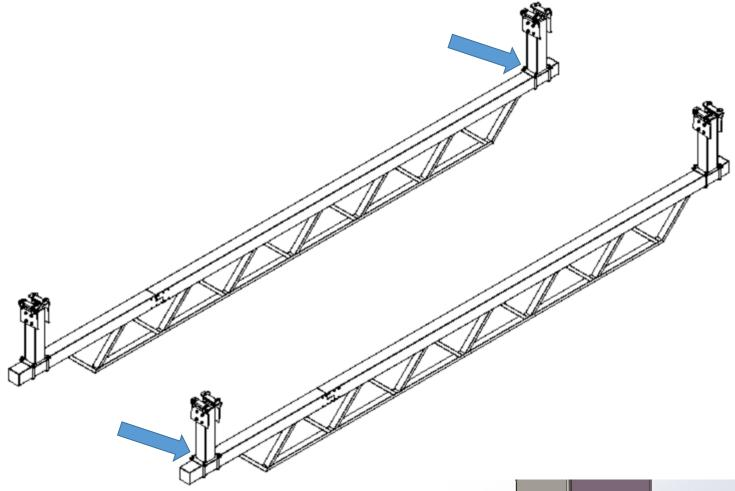
Install the roof beam to 4 hanging pillars by U-shape lock
